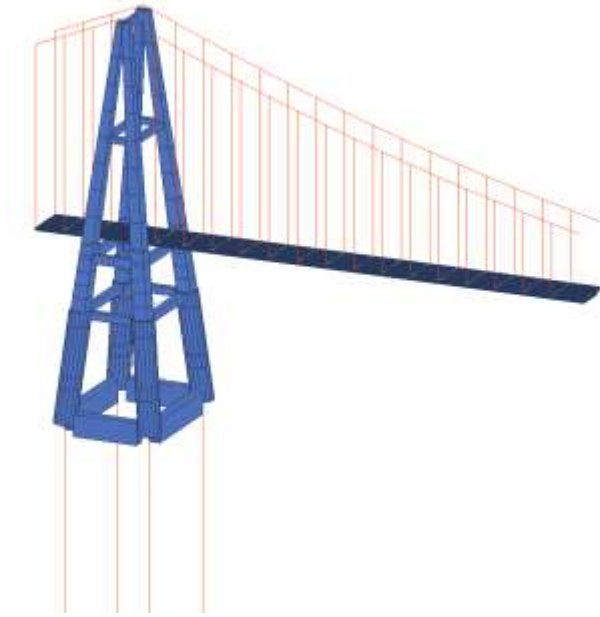
Figure 5. Graphical representation of RM Bridge structural model showing TLP-supported Pylon
