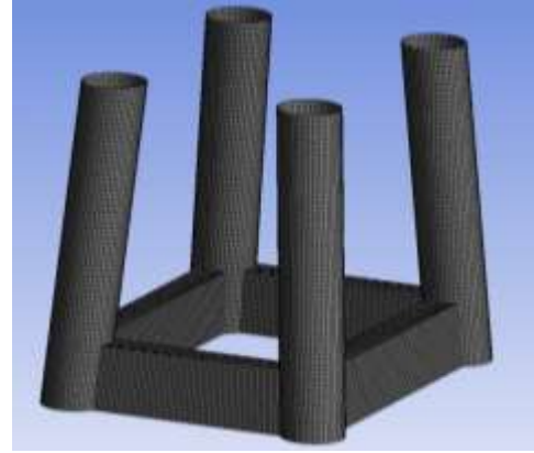
Figure 6. Hydrodynamic panel model developed in Ansys AQWA for obtaining hydrodynamic and hydrostatic properties
