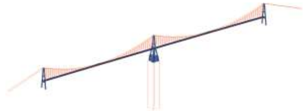
Figure 5. Overview of RM Bridge Analysis model with the 4-legged steel floater concept.
